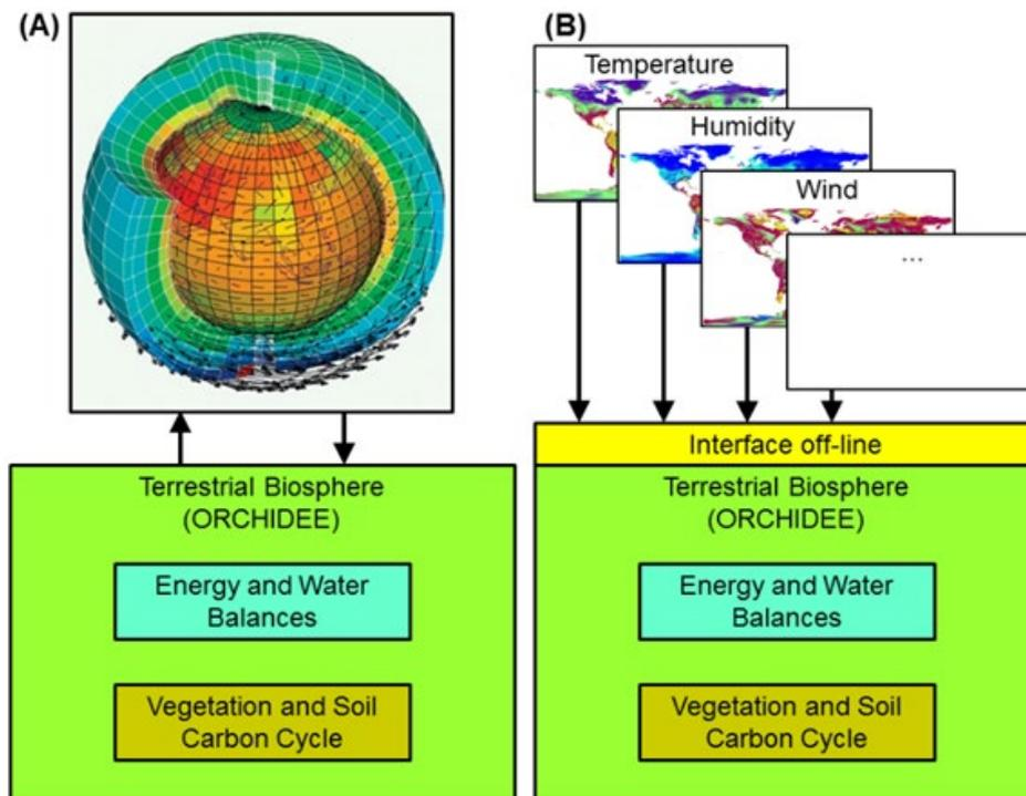
Figure 4.1. Overview of the configurations of the ORCHIDEE model. (A) Shows the coupled configuration in which the two-way interaction between the land and the atmosphere is accounted for. The land surface conditions affect the climate simulations which in turn affect the land surface conditions. (B) the offline configuration in which the climate forcing affects the land surface but the simulated land surface conditions does not affect the climate forcing.
