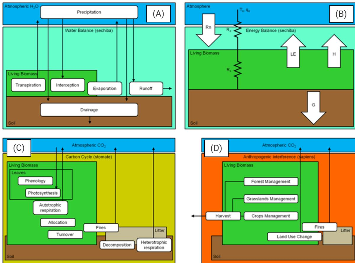
Figure 4.2. Processes represented in the ORCHIDEE model. (A) Main hydraulic processes simulated in ORCHIDEE. (B) Main energy fluxes and pools simulated in ORCHIDEE. (C) Main biogeochemical processes simulated in ORCHIDEE. (D) Main anthropogenic processes simulated in ORCHIDEE.
